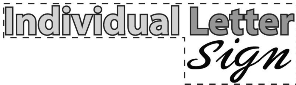
Figure 11-3: Sign Area Measurement (Individual Letter Signs)
