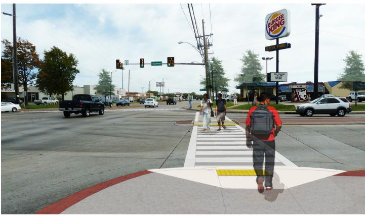
Conceptual photo-rendering of a high visibility crosswalk, re-aligned curb ramp and refuge island median
